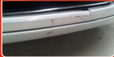
Bumper scratches and crack
